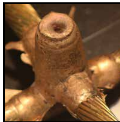
Image 4: Weld is too high. This makes it difficult to remove the weld from the mold.
